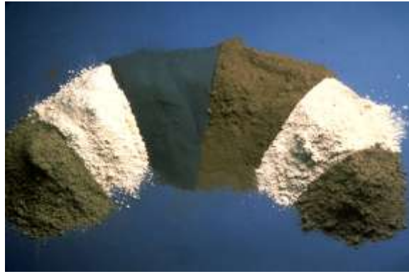
Supplementary cementitious materials. From left to right, fly ash (Class C), metakaolin (calcined clay), silica fume, fly ash (Class F), slag, and calcined shale.
